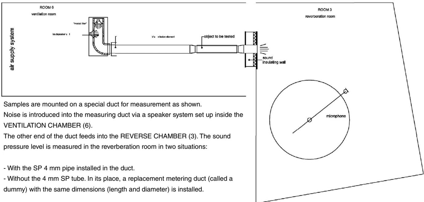
Samples are mounted on a special duct for measurement as shown. Noise is introduced into the measuring duct via a speaker system set up inside the VENTILATION CHAMBER (6).
