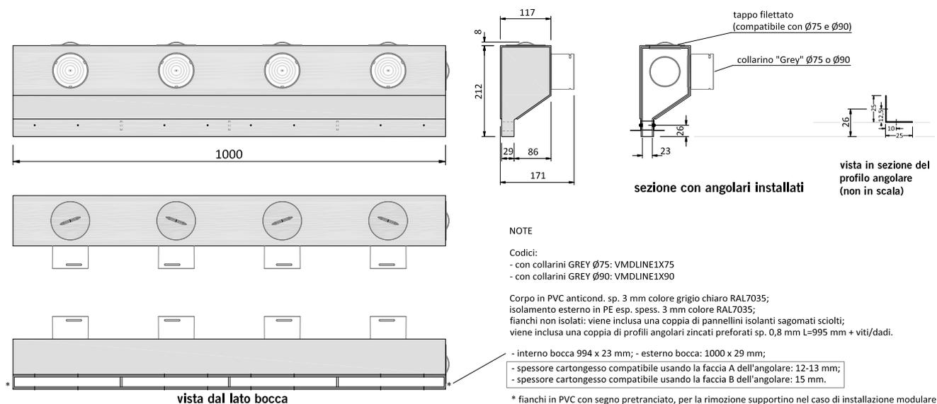
**DIMENSIONI | PLENUM/DIFFUSORE LINEARE MOD. "LINE-S" 500, BOCCA 23, CON COLLARE Ø125 REVERS. COD. VMDLINE235X1125**
