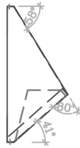
Cross-section drawing of the "cover" of the grille, to be snapped onto the "base"
